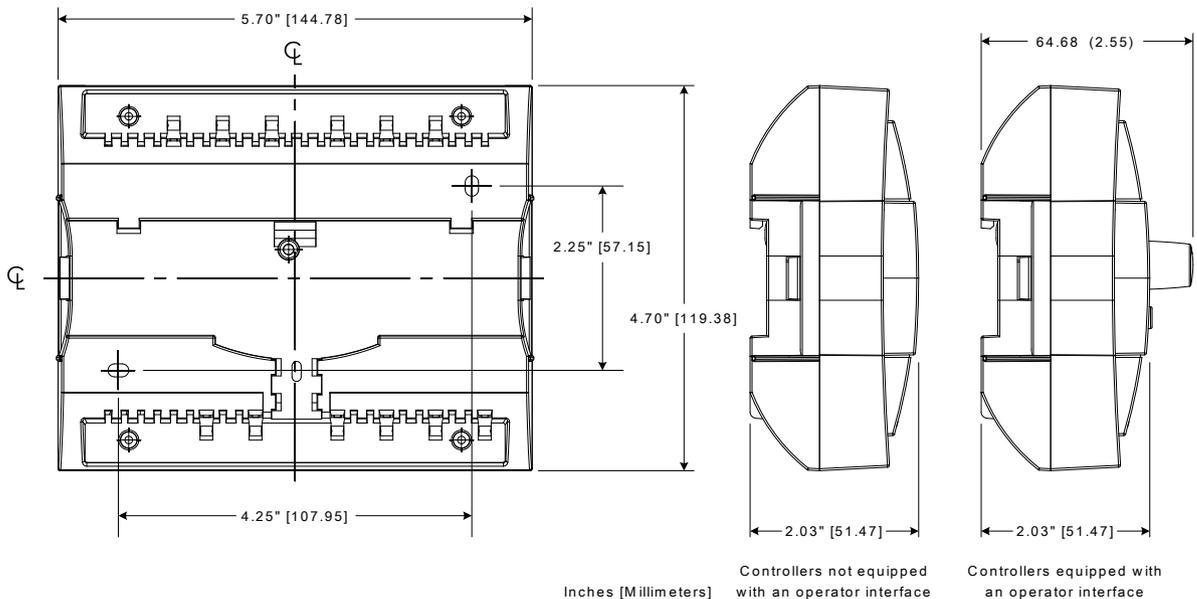
Inches [Millimeters] Controllers not equipped with an operator interface
