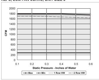
NOTES: VCU or ACU fan speed controller is standard with each unit. Fan curves indicate the maximum and minimum achievable airflows. See Product Description section, page B2-88 for definitions of VCU and ACU controllers. Units must be selected to operate within the airflow and external static pressure ranges shown.
