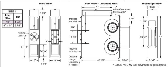
NOTES: Left-hand base unit with electronic control enclosure shown; right-hand is available. See next page for electric heat standard features.
