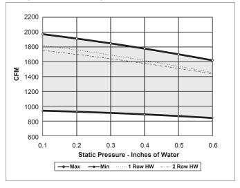
NOTES: Fan speed controller (SCR) is standard with each unit. Fan curves indicate maximum and minimum achievable flow reductions using SCR speed control. Units must be selected to operate within the flow and external static pressure ranges as shown. Fan discharge air volume will be reduced approximately 5% when unit is equipped with optional factory supplied electric heat coils.
