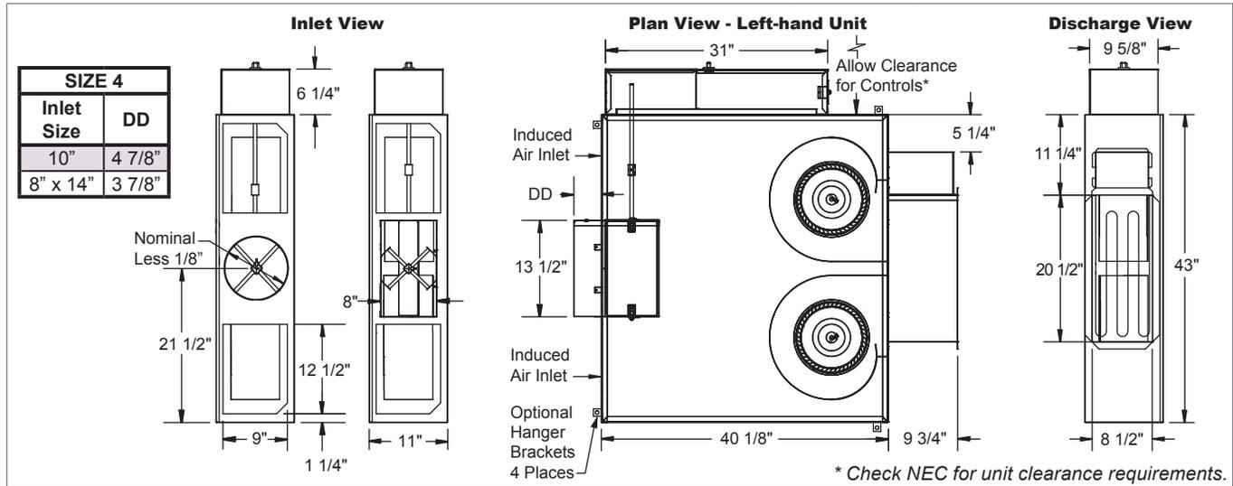
NOTES: Left-hand base unit with electronic control enclosure shown; right-hand is available. See next page for electric heat standard features.
