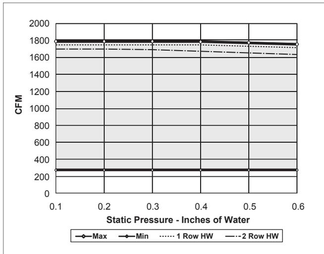
*NOTES: VCU or ACU fan speed controller is standard with each unit. Fan curves indicate the maximum and minimum achievable airflows. See Product Description section, page B2-88 for definitions of VCU and ACU controllers. Units must be selected to operate within the airflow and external static pressure ranges shown.*
