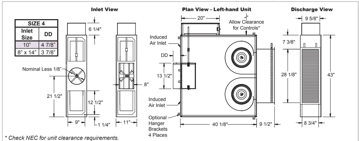
NOTE: Left-hand base unit with electronic control enclosure shown; right-hand is available.
