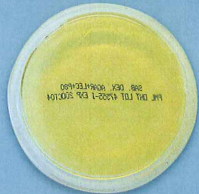
Coil Surface Sample After Installing V-Ray WD
