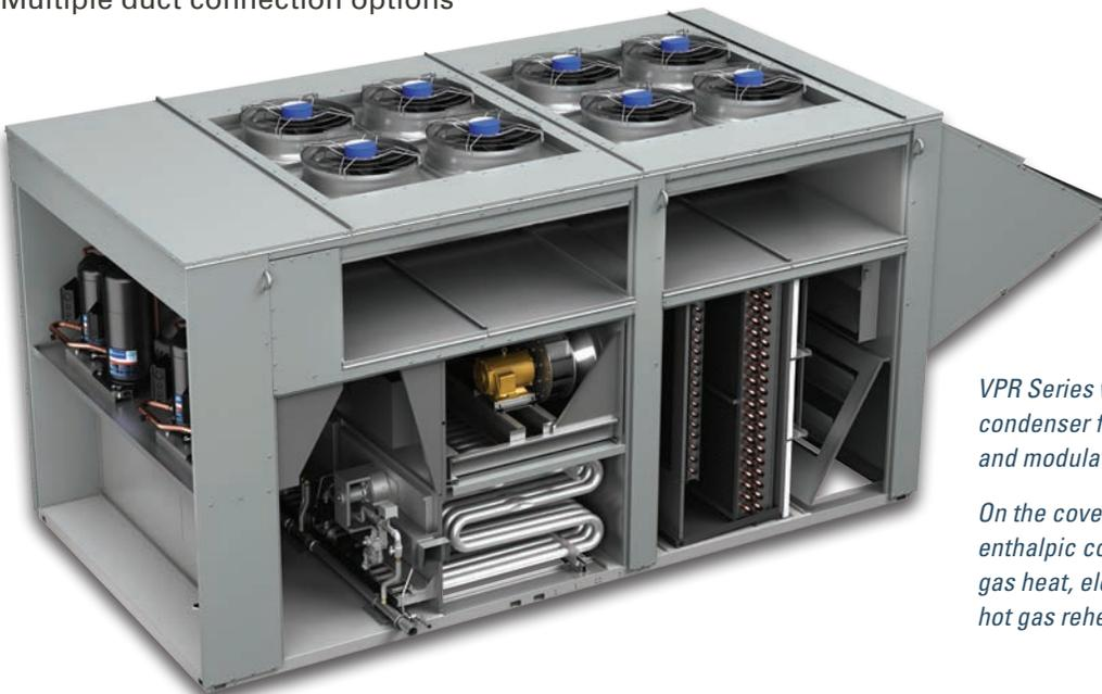
*VPR Series with 352 casing, EC-driven condenser fans, 10:1 turndown gas heat, and modulating hot gas reheat*
