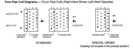
Because of the variations of circuiting available, the location of the inlet and outlet connections may vary up and down. However, always use the following rule to be correct. *The inlet is always the lower connection and the farthest away from the entering-air-side. The outlet connection is always the higher connection closest to the entering-air-side.*
