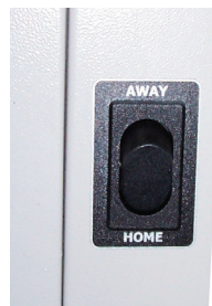
Optional Vacated Premises Selector Switch (Kit# 9WS01)
