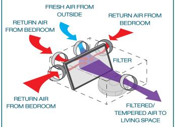
HOW THE BVS120/200 FAN WORKS
