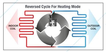
Heat pumps use a reversing valve to reverse the refrigeration system and pull heat from the ambient outdoor air
